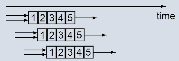
memory access from device memory has a delay of 400-600 cycles; with 40 threads this is equivalent to 10-15 operations, so hopefully there's enough computation to hide the latency
